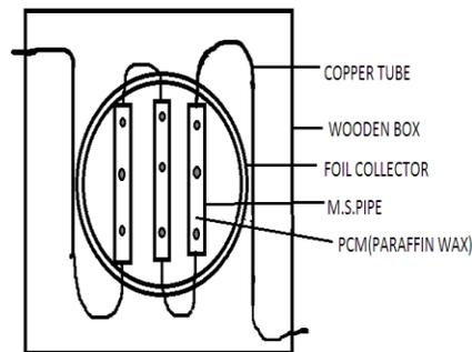
*Fig:3.1 Experimental Set up of Solar Water Heater with PCM*
